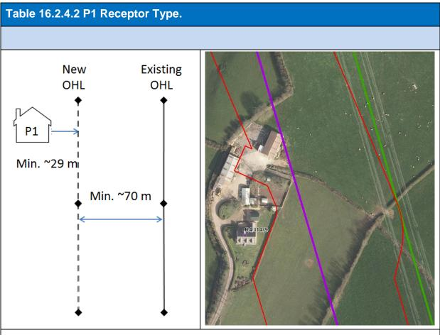
The example above is receptor R4/01479. R4/01479 is approximately 100 m from the existing OHL, shown in green in the image on the right. Option A, shown in purple, would pass between R4/01479 and the exisiting OHL, passing 35 m from the receptor. For Option B (not shown) the new OHL would be closer, passing approximately 29 m from R4/01479.
