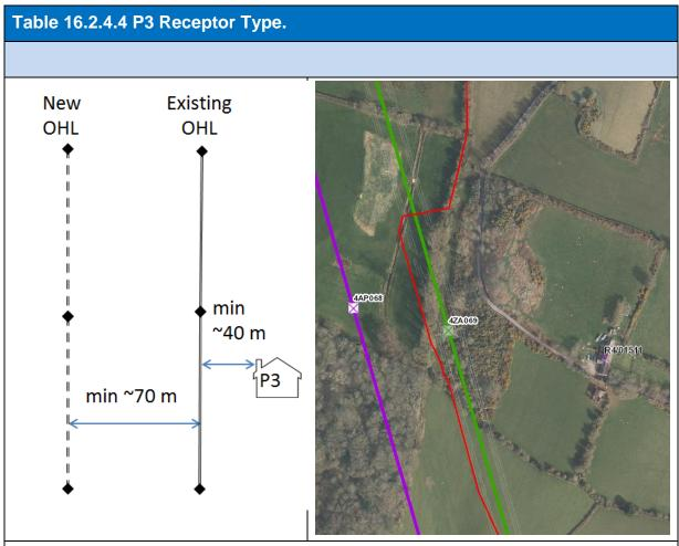
The example above is receptor R4/01511, which is approximately 95 m from the exsiting OHL, shown in green in the image. The new OHL, shown in purple, would pass on the far side of the exisiting OHL and would be approximatley 165 m from R4/01511.
