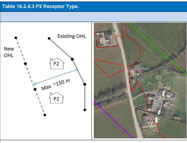
The example above is for the receptors between the old and new OHLs. The southernmost property, R3/13295, would be approximately 30 m from the new OHL to the southwest (purple) and is 100 m from the exsiting OHL (to the northeast, green).
