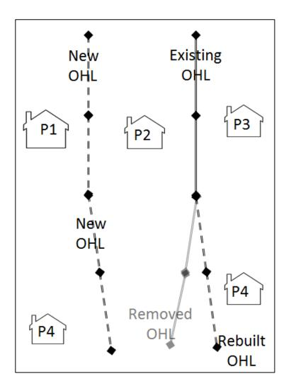
Image 16.2.4.1 Schematic of OHL Parallel Sections
